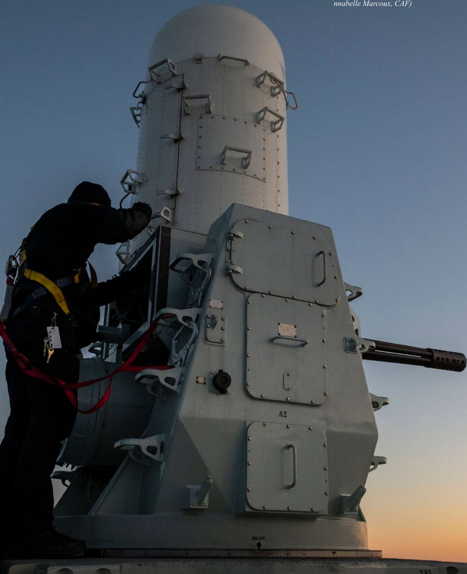
Members of HMCS St. John's doing maintenance on the CIWS (Photo: nnabelle Marcoux, CAF)
